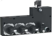
Incorporates up to three electronically controlled pumps, stainless steel valves and moulded plug connections, avoiding any need for wiring in the AHU. As the system operates at low voltage, it is safer for installation or maintenance technicians.
